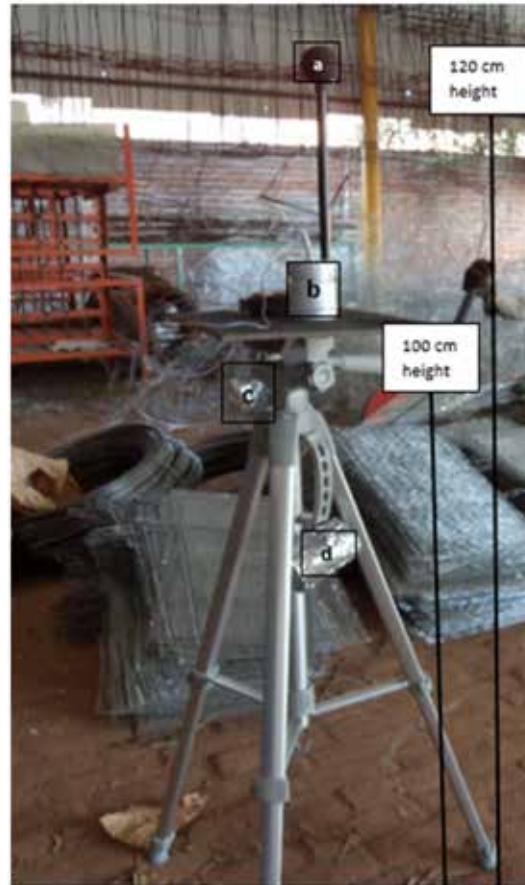
Figure 1. The placement of the equipment to measure the thermal environmental parameters. (a) Sensor to measure the globe temperature T_g , (b) Sensor to measure the wet bulb temperature T_{nw} , (c) Sensor to measure the ambient temperature T_a , (d) EL-USB-2-LCD data logger.
