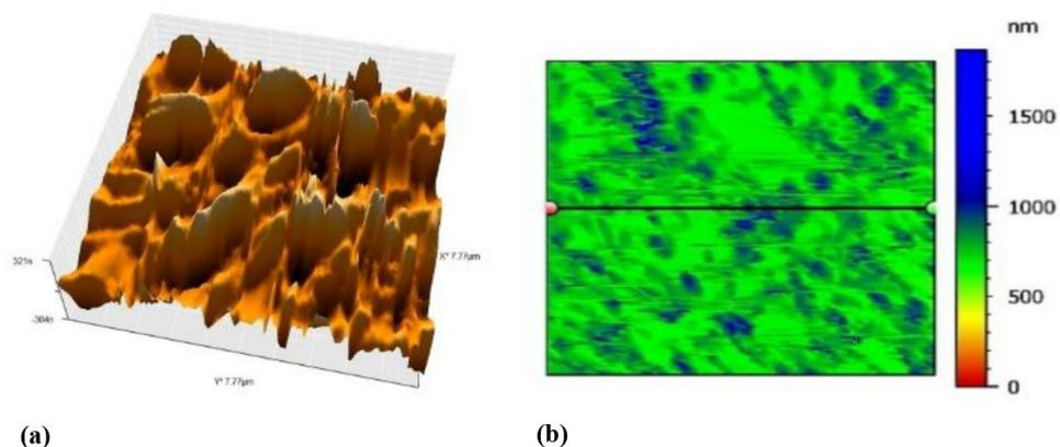
**Figure 3.** Atomic force microscopy (AFM) images of lithium disilicate cylinders (acid etched, Group 2): (a) 3D; (b) pseudo-color view of the surface.
