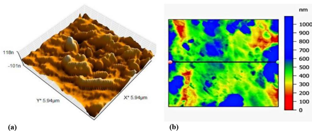
**Figure 4.** Atomic force microscopy (AFM) images of lithium disilicate cylinders (laser irradiated sample power 7 W, Group 3): (a) 3D; (b) pseudo-color view of the surface.
