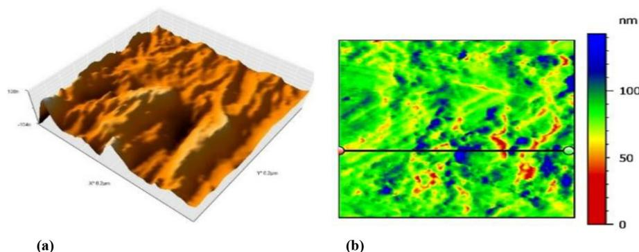
**Figure 2. Atomic force microscopy (AFM) images of lithium disilicate cylinders (untreated, Group 1): (a) 3D; (b) pseudo-color view of the surface.**
