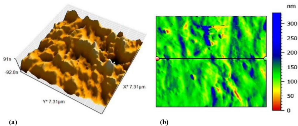
**Figure 5.** Atomic force microscopy (AFM) images of lithium disilicate cylinders (laser irradiated sample power 5 W, Group 4): (a) 3D; (b) pseudo-color view of the surface.
