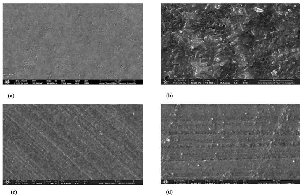
**Figure 6. Scanning electron microscopy (SEM) images of lithium disilicate cylinders at 10000X: (a) SEM of untreated sample, Group 1; (b) SEM of acid etched sample, Group 2; (c) SEM of laser irradiated sample power 5 W, Group 4; (d) SEM of laser irradiated sample power 7 W, Group 3.**
