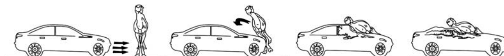
Figure 2. How collision with a camel results in the animal falling on and through the poorly reinforced frontal section of the car's upper surface (roof and windshield) usually with severe consequences to the occupants of the front seat.
